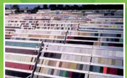
Testing component elements in genuine conditions, in an outdoor laboratory in Florida
